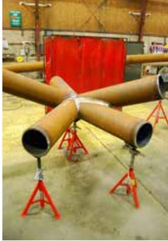
◀ An inside look at one of the waterfall node castings (left) and connecting a node to five round HSS (right). A combination of fillet and partial-penetration welds were used to complete the connections at each steel node casting.
